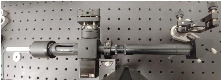
Figure 9: Picture of the assembled compact interferometer, which is mounted in front of a flat mirror visible in the top-right.
