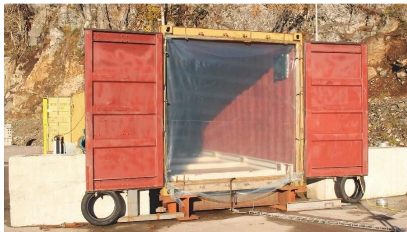
Figure 7: Container doors in fully open position, and opening covered by a polyethylene sheet.
