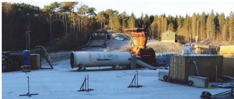
Figure 2: Test site with a 20-foot container and supports for the three external pressure sensors. 2
