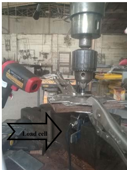
Fig. 6 Load cell and infrared temperature device arrangement
