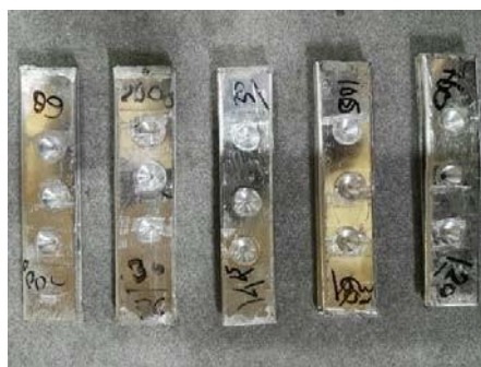
Fig. 11 Surface flash removal
