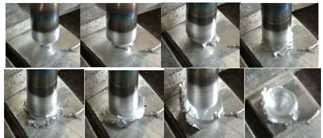
Fig. 8 Sequence of FSSW for AA1100
