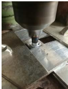
Fig. 5 Welding pin fixation in drilling holder
