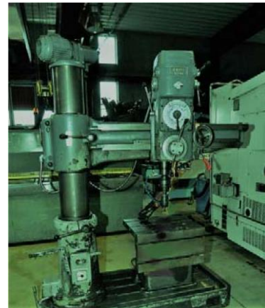
Fig. 2 Drilling machine, type Breda R915L
