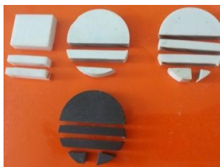
Fig. 6 Corundum ceramics materials with different compositions and experimental specimens fabricated from them
