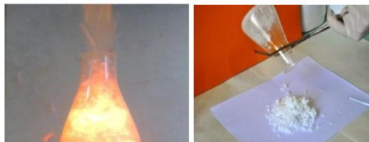
Fig. 1 Obtaining \alpha -Al 2 O 3 powder from (NO 3 ) 3 -NH 2 CONH 2 compound by oxidation-reduction reaction
