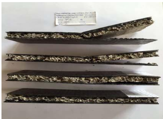
Fig. 6 Collapsed sandwiches named E1.5A10 after the bending tests at different support span values (top to bottom: L = 55, 70, 80 and 125 mm)
