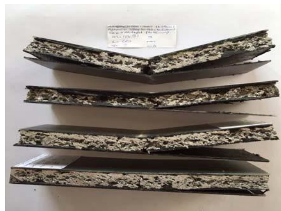
Fig. 9 Collapsed sandwiches named S1.5A15 after the bending tests at different support span values (top to bottom: L = 55, 70, 80 tests and 125 mm)
