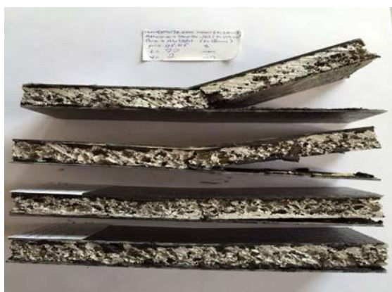
Fig. 7 Collapsed sandwiches named E1.5A15 after the bending at different support span values (top to bottom: L = 55, 70, 80 and 125 mm)
