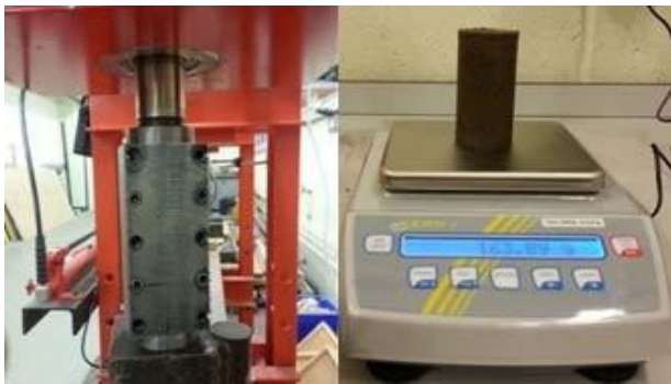
Fig. 7 Hydraulic Compaction and Weighing of a Specimen during Specimens Preparation
