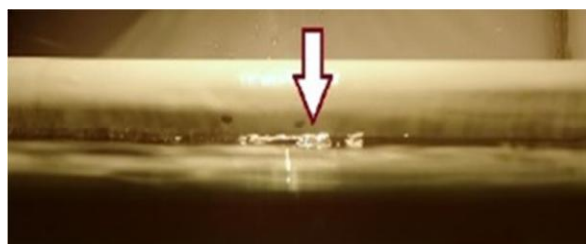
Fig. 4 Front view of the cylinder showing Water Chute in Air medium
