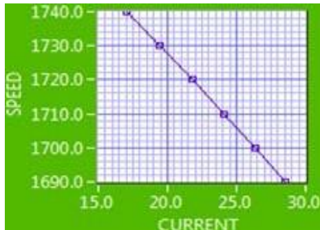
Fig. 6 Speed vs current of induction motor
