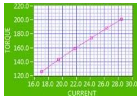
Fig. 5 Torque vs current characteristics of induction motor
