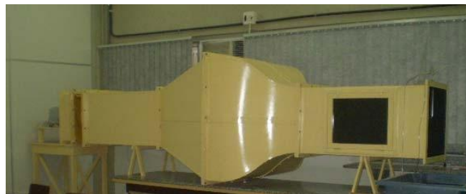
Fig. 10 Tunnel of installed wind
