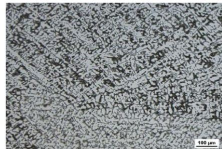
Fig. 1 The α-phase in secondary AlSi9Cu3 cast alloy, as-cast state. Optical microscope, etch. H 2 SO 4
