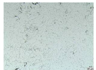
Fig. 7 (b) Optical micrograph of as-cast 7075 (alloy B)
