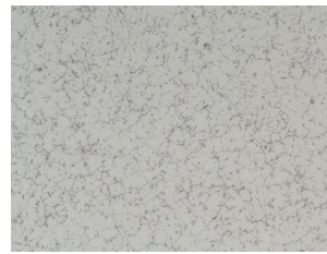
Fig. 7 (c) Optical micrograph of as-cast 7075 (alloy C)
