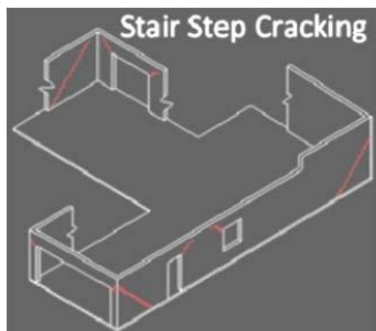
Fig. 1 Stair Step Crack Mapping
