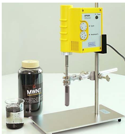
Fig. 8 Ultrasonic Dispersion of CNTs [16]
