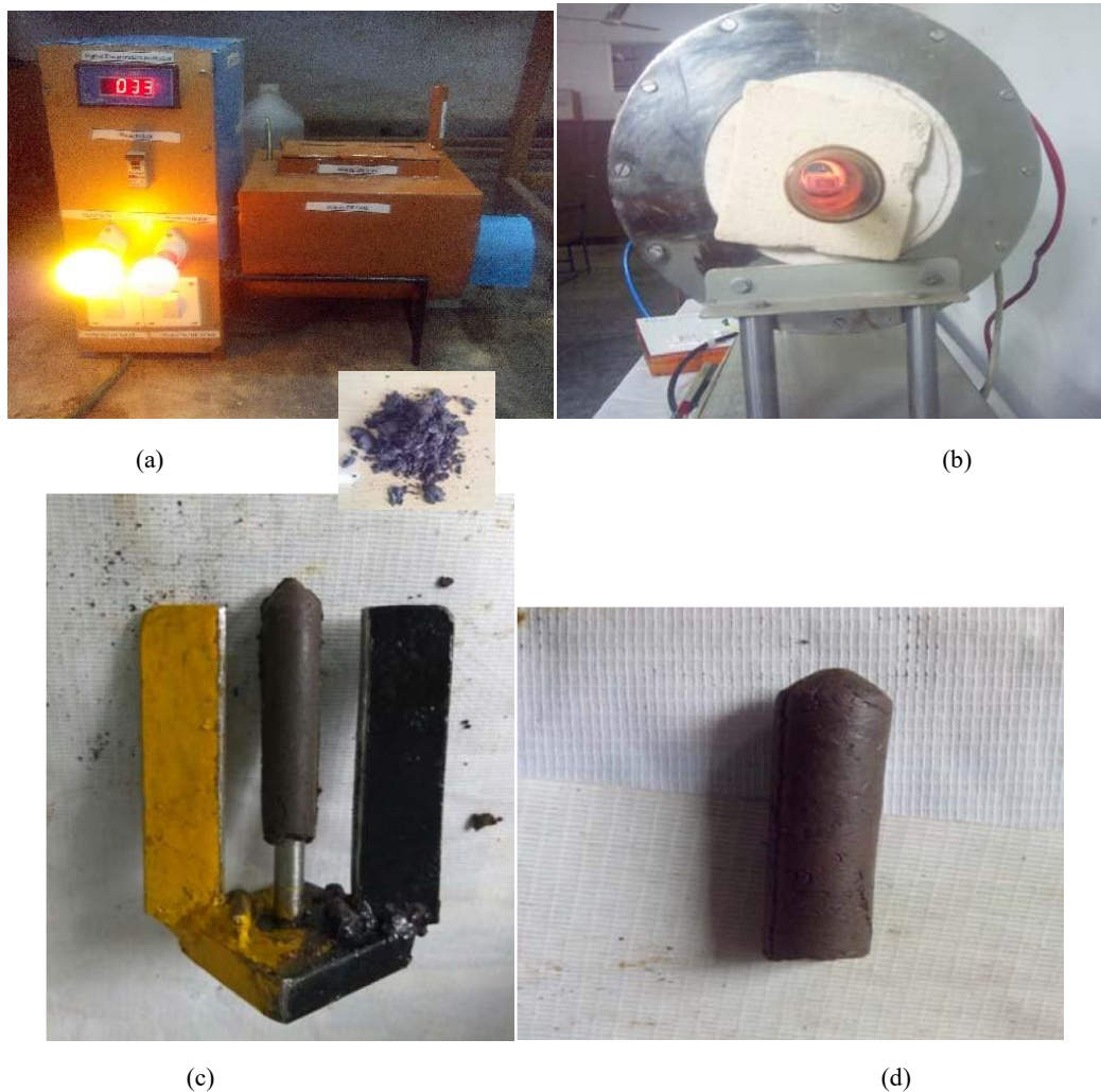
Fig. 4 (A) Fabricated sigma mixer with Green Mixture, (B) Schematic diagram of furnace used for sintering, (C) Green filter sample with dies
