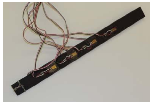
Fig. 3 Test specimen for measuring bending stresses
