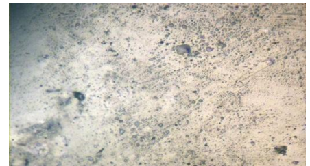
Fig. 19 Micrograph of 15% cow bone filler
