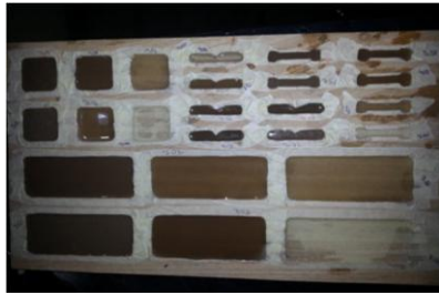
Fig. 4 Mould filled with CBRPC samples
