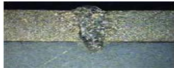
Fig. 1 Lap joint between Al 6082 and Ti G2
