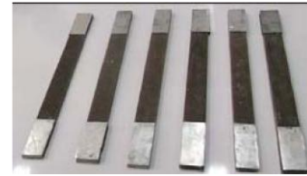
Fig. 2 Samples jute/epoxy reinforcement fabric of jute
