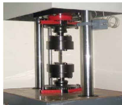
Fig. 4 Fatigue test of the laminate
