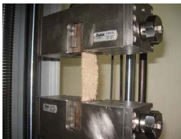
Fig. 1 Tensile test of the jute fabric
