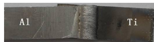
Fig. 8 Fracture location of tensile test
