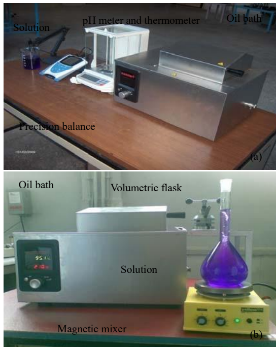
Fig. 2 The equipment for electroless Ni-B deposition
