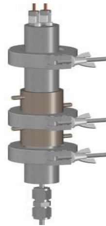
Fig. 4 The combination diagram of vacuum inhalation chamber
